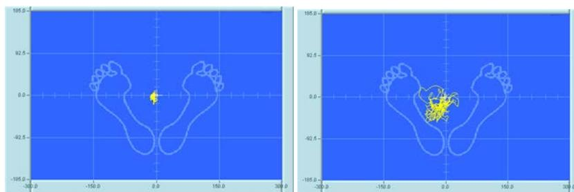
Figure 3. **Left:** recording of the displacement of the centre of pressure of a person with stable balance. **Right:** recording of a more unstable person. The displacement or sway of the centre of pressure is greater.
