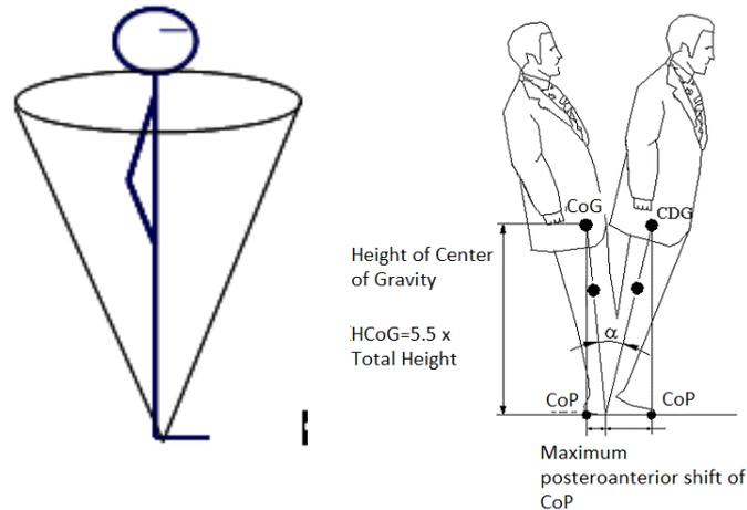
Figure 1. Inverted pendulum model and calculation of the displacement of the centre of pressure according to the height of the person being assessed.
