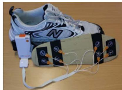
**Figure 2.** Instrumented insole. Image from the article by Davies RJ et al., 2016
